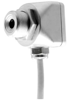
Model TB-2000LT-SFA2 is a compact on-line infrared thermometer for non-contact temperature measurement in the range of 0 to 500°C. It provides linear 4~20mA output (2-wire) as well as TTL interface for external display, recording or data-processing. Both analog and digital outputs can be utilized simultaneously.
